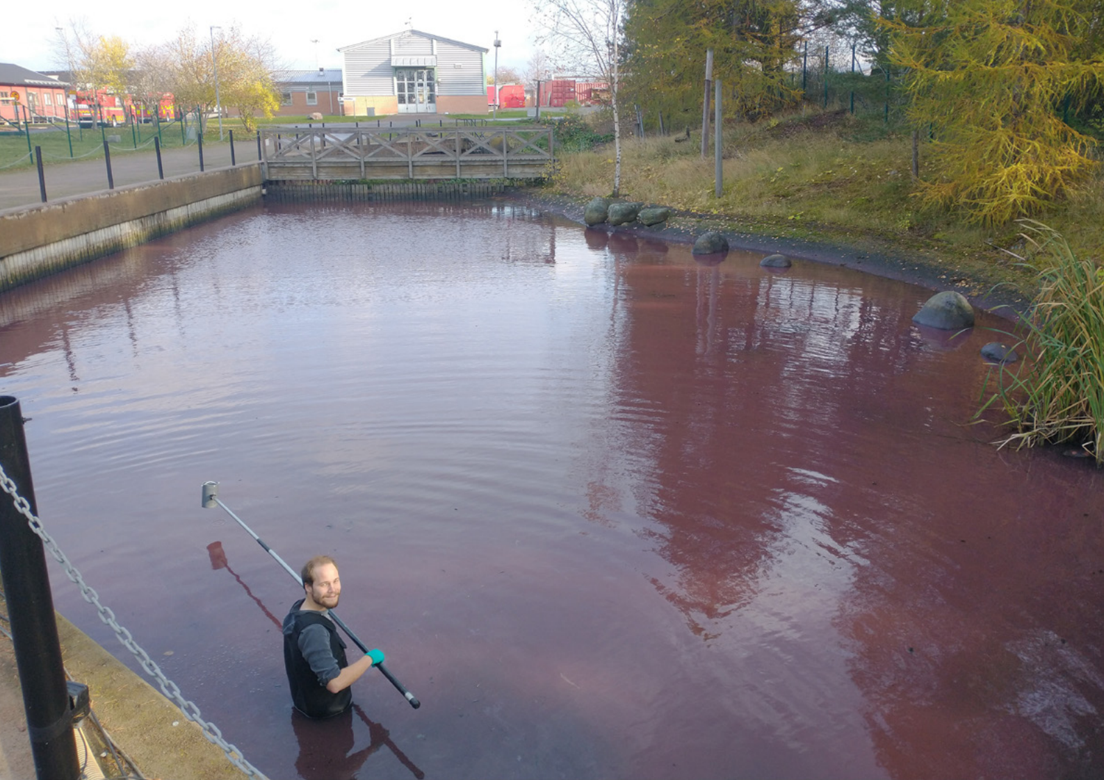
Sampling of an aqueous film forming foam (AFFF) contaminated pond at Viktoria Fire Fighting Training Site, Uppsala, Sweden.
